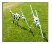
Frequent realignment of the instruments and zero drift correction ensure a constant high quality of data. Extremely sensitive, these instruments can detect variations in soil magnetism to 0.1nT, affording diverse application throughout a variety of archaeological, soil morphological and geological conditions.
